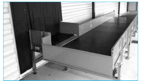
Conveyor for deposit or baggage claim
