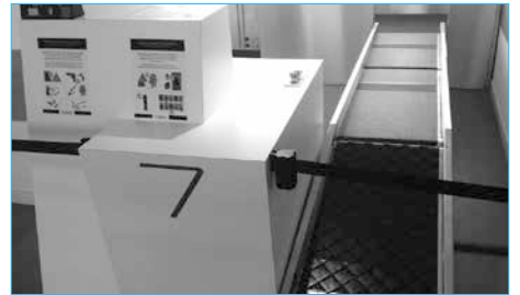
Standard baggage check-in conveyor (3 belts)
