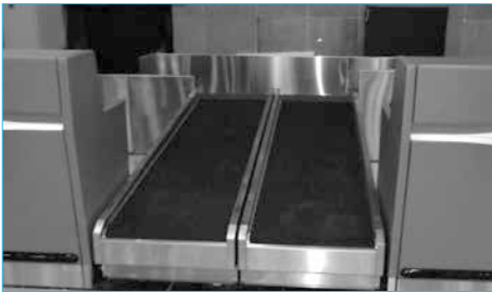
Standard baggage check-in conveyor (1 belt)
