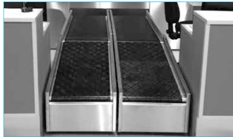
Standard baggage check-in conveyor (2 belts)
